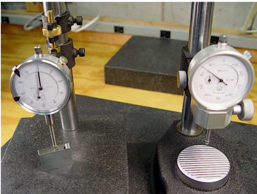
Fig. 2. Differential measurements with comparator dial and block gauges.
