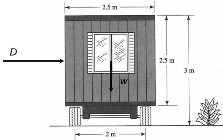
Assume center of gravity is at center of home. When overturning is imminent, no weight is on the right wheel. Then taking moments ( $M$ ) about the right wheel:
