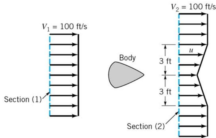
5.23 The results of a wind tunnel test to determine the drag on a body (see Fig. P5.23) are summarized below. The upstream [section (1)] velocity is uniform at 100 ft/s. The static pressures are given by  $p_1 = p_2 = 14.7$  psia. The downstream velocity distribution which is symmetrical about the centerline is given by
