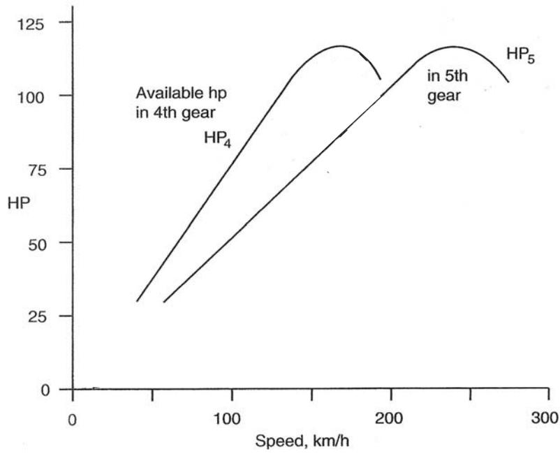
The maximum steady-state speed of a vehicle is achieved when the maximum available driving force at that speed equals the resistance force due to aerodynamic drag and tire resistance.
