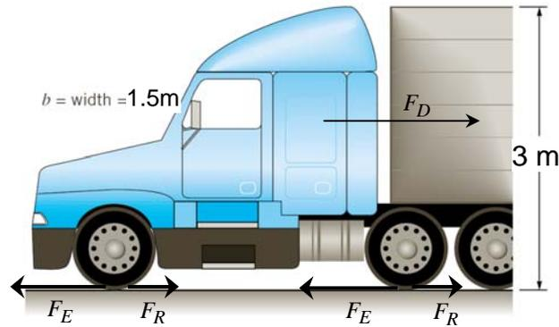
The truck is moving at constant speed, hence the sum of forces acting on the truck must be zero. There are three forces acting on the truck, the Drag Force  $F_D$ , the Rolling Resistance  $F_R$  and the Forward Force from the engine through the wheels  $F_E$ .
