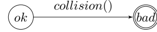
Fig. 6. The observer automaton checking for collisions in the system. The function collision() is described in section VI.
