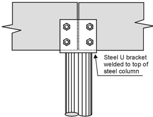
Figure 6.19: Beam to steel column detail.
