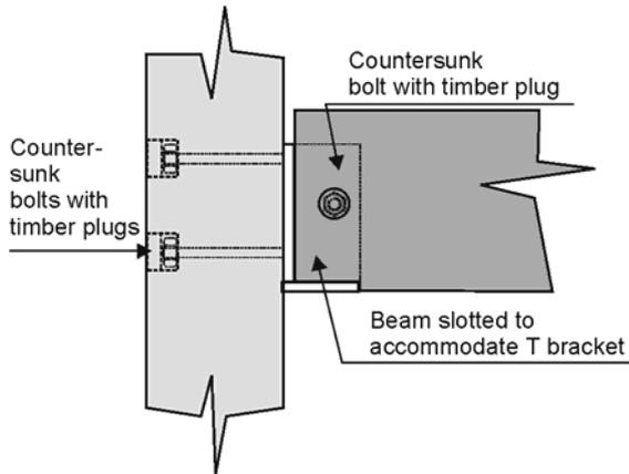
Figure 6.21: Beam to column connection, where the connectors have been recessed and are hidden.
