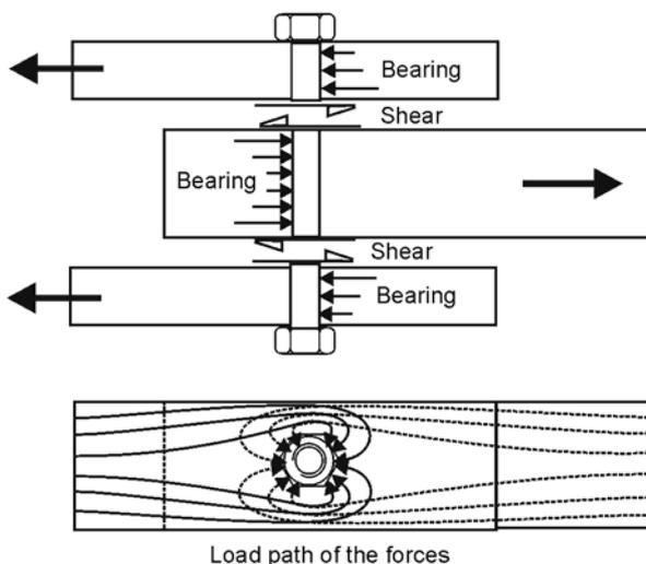
Figure 6.5: Bolted connection showing the convoluted load path for the transfer of the forces.
