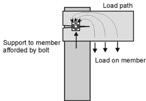
Figure 6.2: Loading of member in tension. Cracking may occur when end distance is insufficient.
