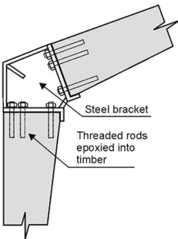
Figure 6.39: Eaves joint for portal frame. Steel bracket makes it possible to assemble the joint on site. Threaded rods must be glued under factory conditions.
