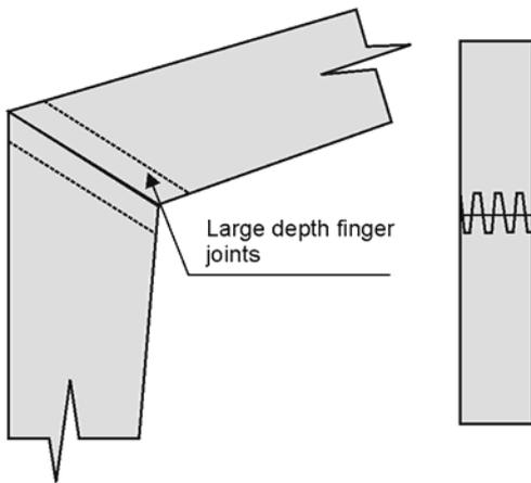
Figure 6.41: Eaves joint manufactured by using large finger joints.
