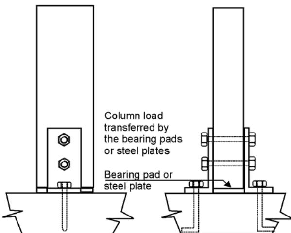
Figure 6.9: Transfer of loading through bearing pads.
