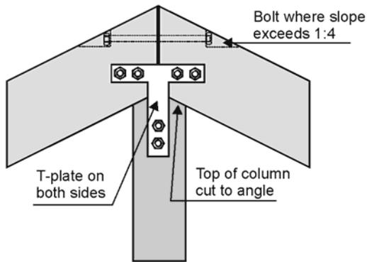
Figure 6.18: Beam to column detail where the beams are pitched.
