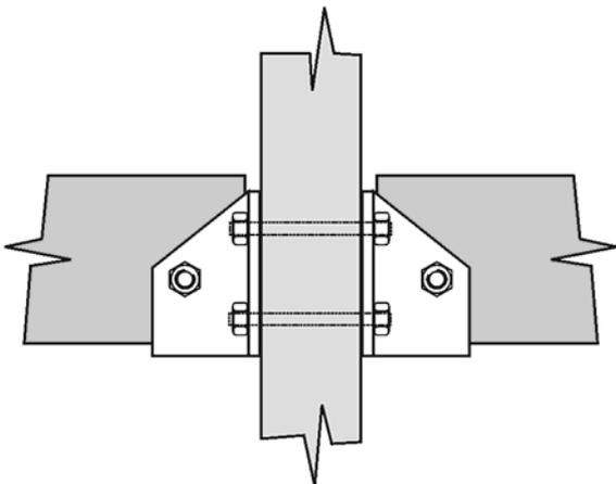
Figure 6.20: Beam to column connection where the column is continuous past the beam level.
