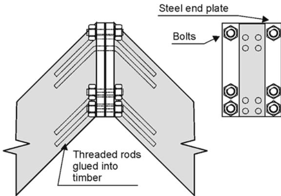
Figure 6.37: Moment connection using threaded rods and steel end plates. Rods can be threaded into the steel plates and then bent, or simply welded onto the end plates. Connection can be assembled on site.
