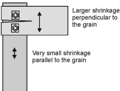
Figure 6.1: Splitting of timber as a result of differential shrinkage.
