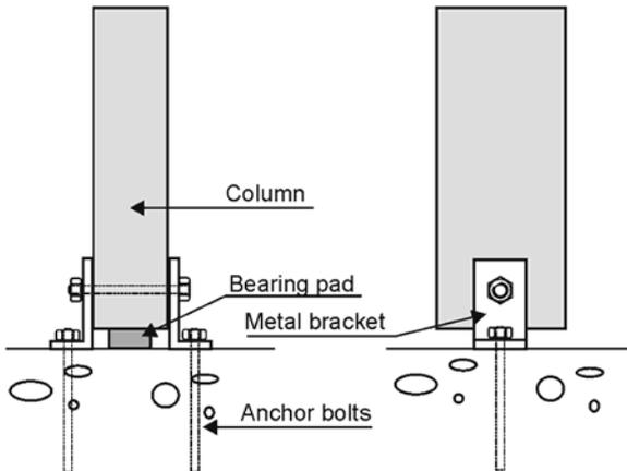
Figure 6.13: Column base with two angle brackets, force transfer through bearing on pad.
