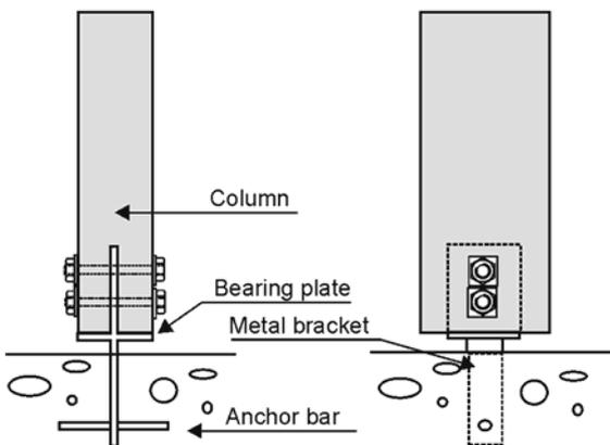
Figure 6.14: Column base with cruciform bracket slotted into the timber. Force transfer through direct bearing on metal plate.
