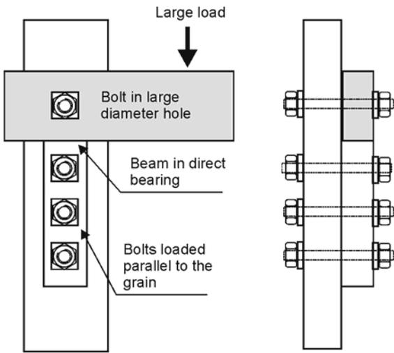
Figure 6.7: A method of avoiding splitting as a result of large tension perpendicular to the grain.
