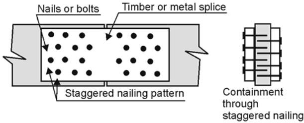
Figure 6.28: Splicing of member that must transfer bending moment and shear.
