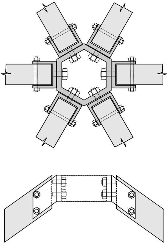
Figure 6.38: Compression ring for apex of dome type structure. Note that a certain amount of moment transfer is possible.
