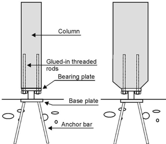
Figure 6.15: Column base with anchor bolts glued into timber column. Force transfer through direct bearing on metal plate.
