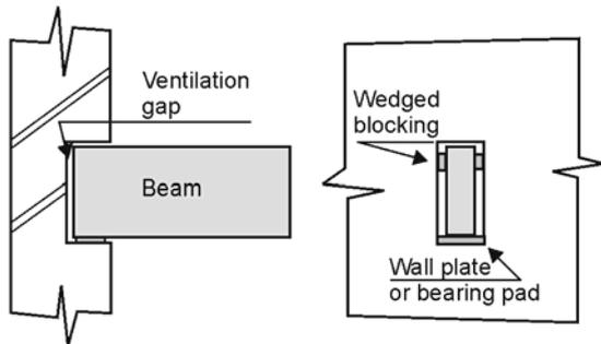
Figure 6.24: Beam built into brick wall with wedged blocking to improve torsional restraint.
