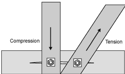
Figure 6.3: Cleaving of member as a result of tension perpendicular to the grain.
