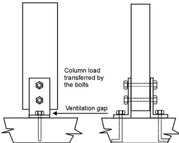
Figure 6.8: Air gap to prevent ingress of moisture into end-grain of column.
