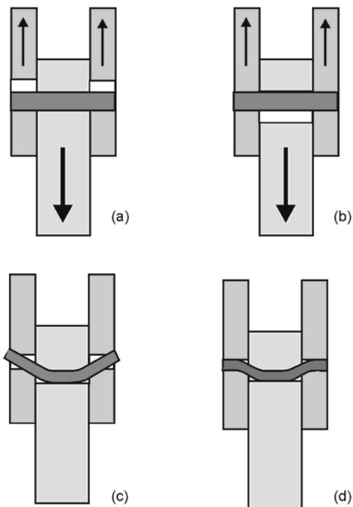
Figure 6.12: Failure on connections and connectors in double shear.
