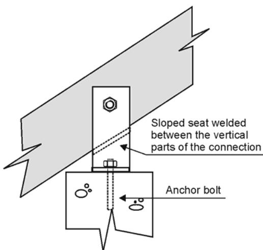
Figure 6.23: Connection for sloped beam.
