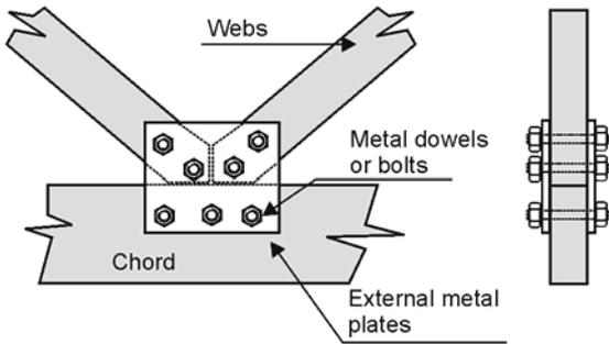
Figure 6.32: External plate connection for members with limited width.
