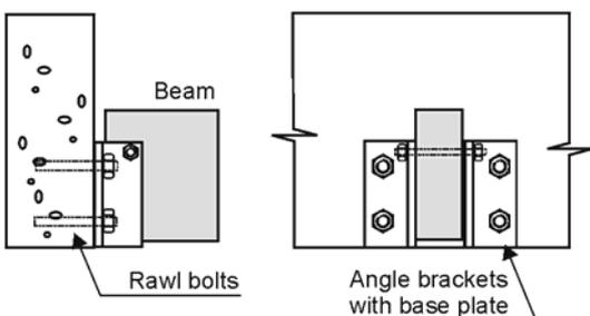
Figure 6.27: Timber beam to concrete beam or wall. It is preferable to transfer load in direct bearing.
