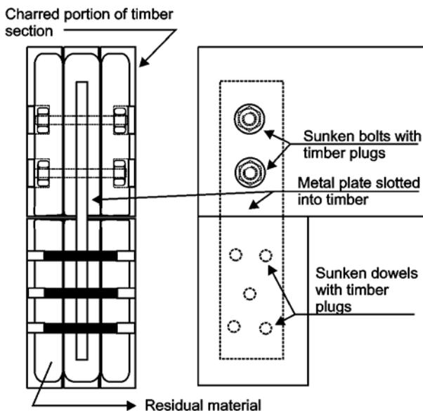
Figure 6.10: Protection of metal connection to achieve the required fire rating.
