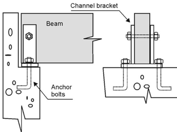
Figure 6.22: Beam to concrete connection. Channel bracket may be used to improve lateral torsional restraint at the support.
