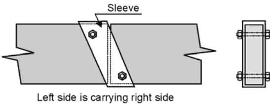
Figure 6.29: Splicing of beams when only shear force must be transferred between the right hand side and the left.
