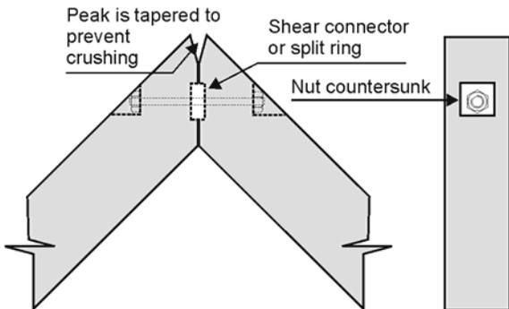
Figure 6.35: Pinned connection, using a shear plate or split ring to transfer the shear.
