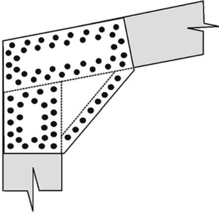
Figure 6.40: Eaves joint using plywood on either side and nailing.
