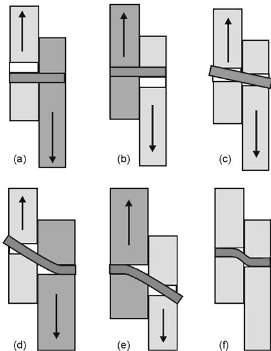
Figure 6.11: Possible failure mechanisms for nails, dowels and bolts.
