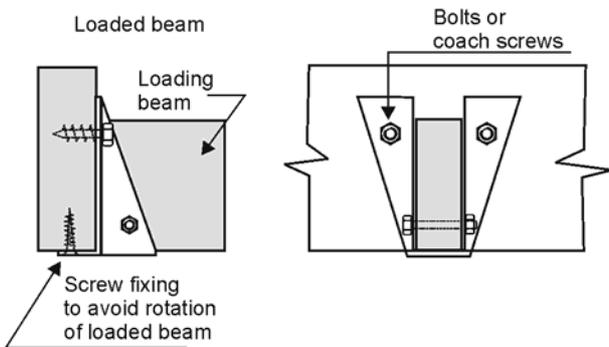
Figure 6.25: Force transfer in direct bearing and through coach screws or bolts. Note that rotation of loaded beam is prevented.
