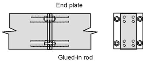
Figure 6.30: Splicing of members with glued-in threaded rods and end plates. Note that this method should not be used where large moisture content variation is expected.
