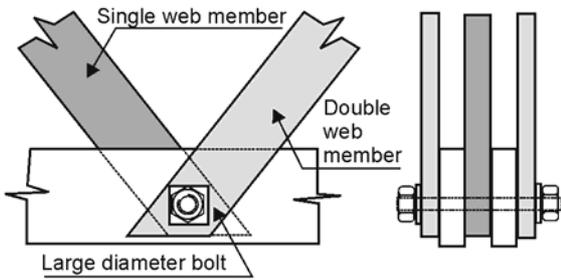
Figure 6.33: Spaced chords where, where the resultant forces lie in the same plane. Large diameter bolts or shear plates and split rings may be used.
