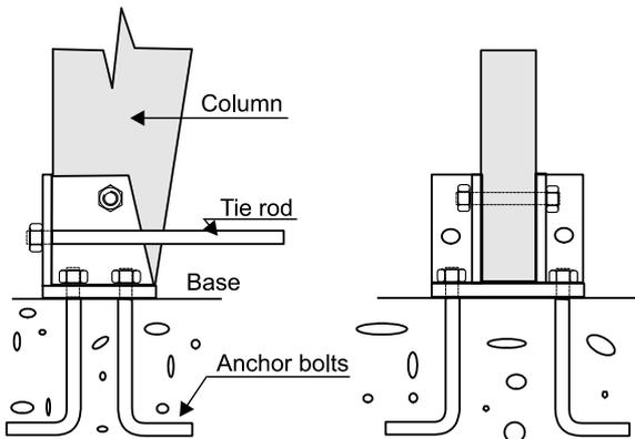
Figure 6.16: Arch or portal frame base plate with tie rod. Tie rod can be covered by an elevated timber floor.
