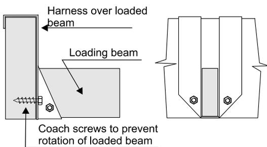
Figure 6.26: Harness over loaded beam, all loads transferred by direct bearing.
