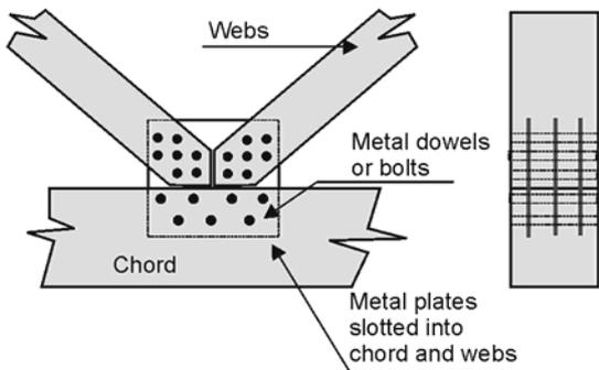
Figure 6.31: Metal plates slotted into the timber members. Connection completed by using metal dowels in tight fitting holes, or bolts.
