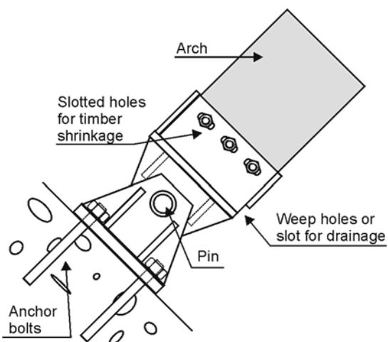
Figure 6.17: Pinned base for an arched structure.
