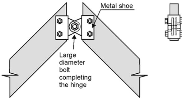
Figure 6.34: Hinged apex connection for a portal frame.
