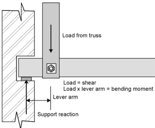
Figure 6.4: Shear force and bending in member as a result of an eccentric connection and support.
